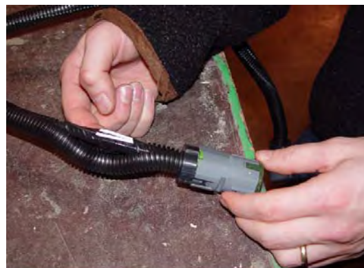
Transmission Connector VIW-V and Harness showing wire 167
