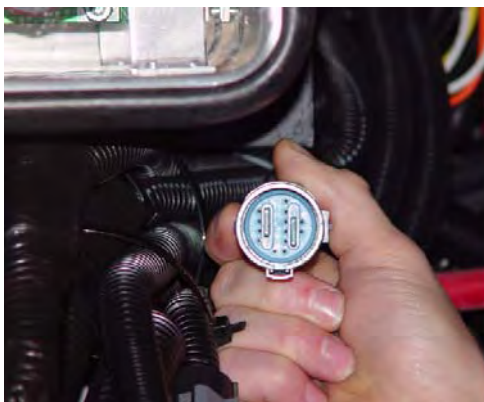
Transmission Connector VIW-V and Harness showing wire 167
